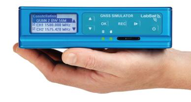
LabSat 3 Wideband greatly increases GNSS Record and Replay capabilities
